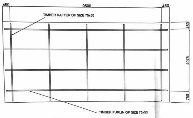
Plan of Roof at security barack near Power House Stage-I All dimensions are in mm
